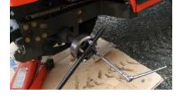
$\triangle$ Please take the time to make the install in 3 steps. First hand tightens the bolts; Second torque the bolts to half the torque in a crisscross pattern & <a href="mailto:finally">finally</a> torque the bolt to their final value of 90 ft-lbs.
